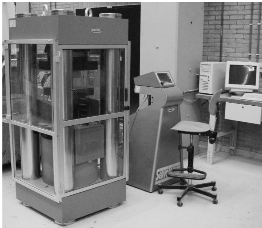
Figure 3 Experimental testing device for concrete compression
