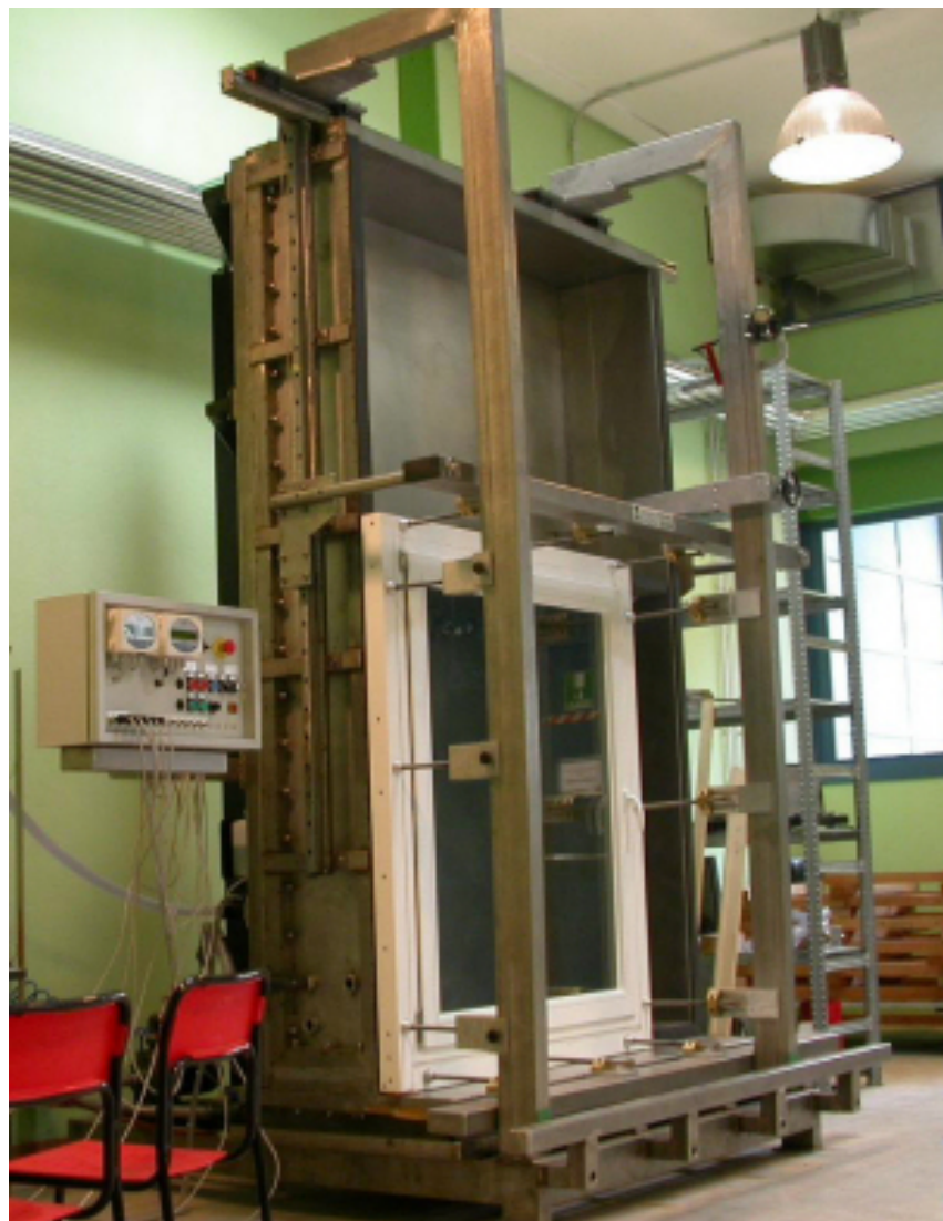
Figure 6 Experimental testing device for measuring the window performance 'Resistance to wind-load' (© ECWINS Consortium)
